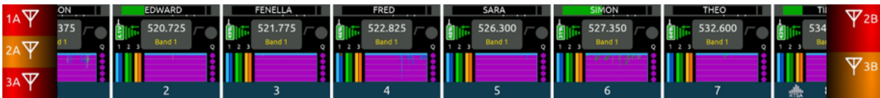
8RX View showing Antenna 2A and 3B approaching overload and Antenna 1A, 3A, and 2B overloading
