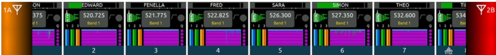
8RX View showing Antenna 2A and 3B approaching overload and Antenna 1A, 3A, and 2B overloading
